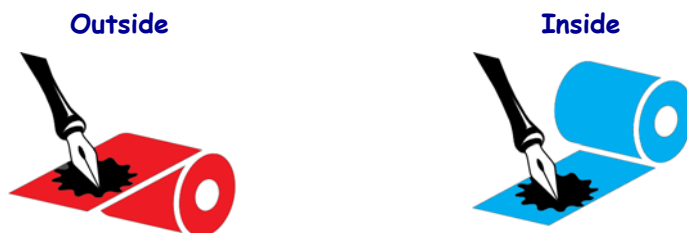
Figure 7 • Ribbon Coated on Outside or Inside
