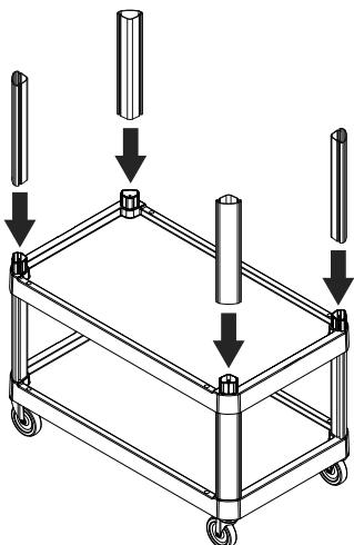
5. Tap supports onto middle shelf using rubber mallet.
