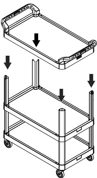
7. Tap top shelf onto supports using rubber mallet. (See Figure 7)
