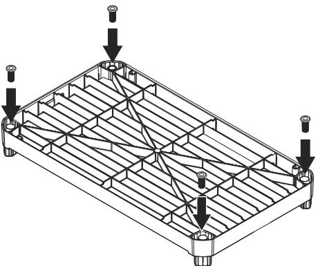
1. Insert caster sockets into each corner of shelf and tap in with rubber mallet until secure. (See Figure 1)
