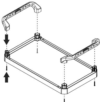
6. Tap handles onto top shelf using rubber mallet. Insert screws into underside of top shelf and secure handles using Phillips screwdriver. (See Figure 6)
