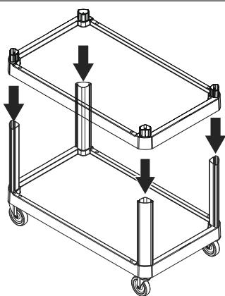
4. Tap middle shelf onto supports using rubber mallet.
