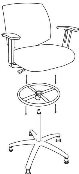
5. Slide footing onto gas lift and tighten knob to secure. (See Figure 5)
