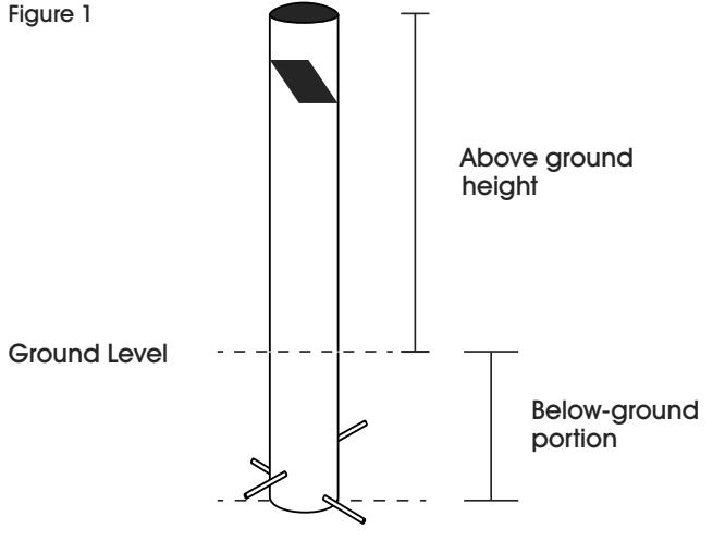
2. Dig a hole for the below-ground portion. Remove a 20 x 20 x 20" cube. This will contain the concrete that will fix the bollard in position. (See Figure 2)
