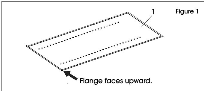
**NOTE:** When bolting the unit together, leave the bolts slightly loose until step 7, unless otherwise specified.
