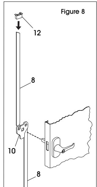
4. Hold the lock bars in position while sliding the lock bar guides (12) over the lock bar ends of the bars and through the door slots. (See Figure 8)
