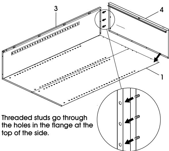
2. Attach the left side (3) to the back by placing flange around the back and bolting the back and sides together. Be sure that the shelf supports on all shelf adjustment strips point up on both back and side. (See Figure 2)
