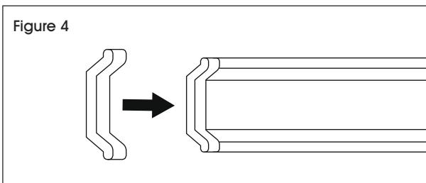
5. Insert the aluminum rail into mounting brackets. Secure the rail by installing the mounting bracket clips. (See Figures 5-6)
