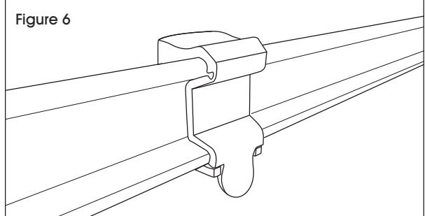
6. Attach grippers to rail by securing the top and then pressing down on the bottom until it clicks. (See Figures 7-8)
