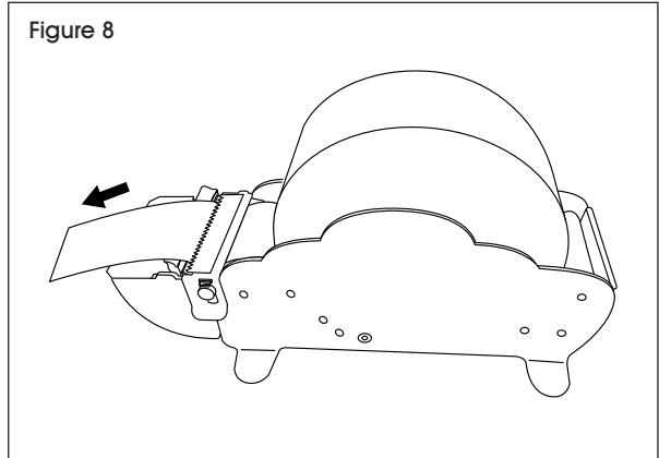
2. When tape is at desired length, pull up against blade to tear tape from roll.
