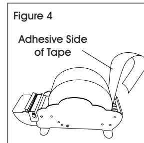
3. Insert tape end in back of two rollers. Push tape through the underside of the dispenser until the end comes out in front of the tape cradle. (See Figure 5)
