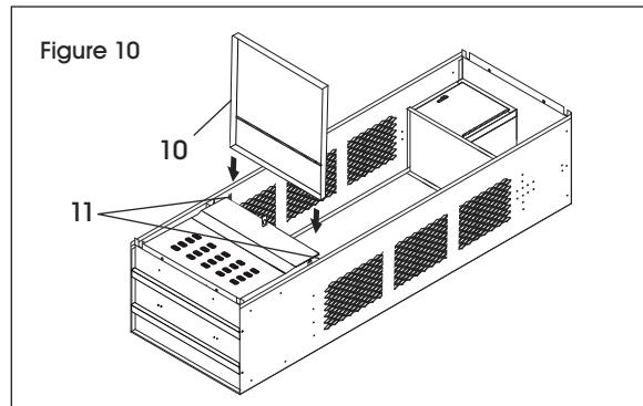
12. Bolt smaller, rectangular panel of the foot locker cover (10) to the foot locker rails (11) on both sides. The padlock hasp on the foot locker cover (10) should align with the hasp on the foot locker front (9). (See Figure 11)
