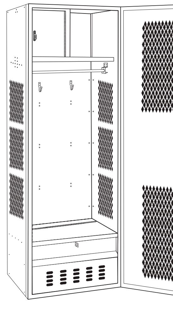
16. Bolt one coat rod bracket (14) to one of the sides (2). Then, insert coat rod (13) into the coat rod bracket (14) that is bolted to the side (2). Place second coat rod bracket (14) over the other end of the coat rod (13). Bolt second coat rod bracket (14) to the other side (2). (See Figure 14)
