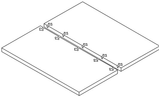
2. Push top sections together so surface sides are flush
