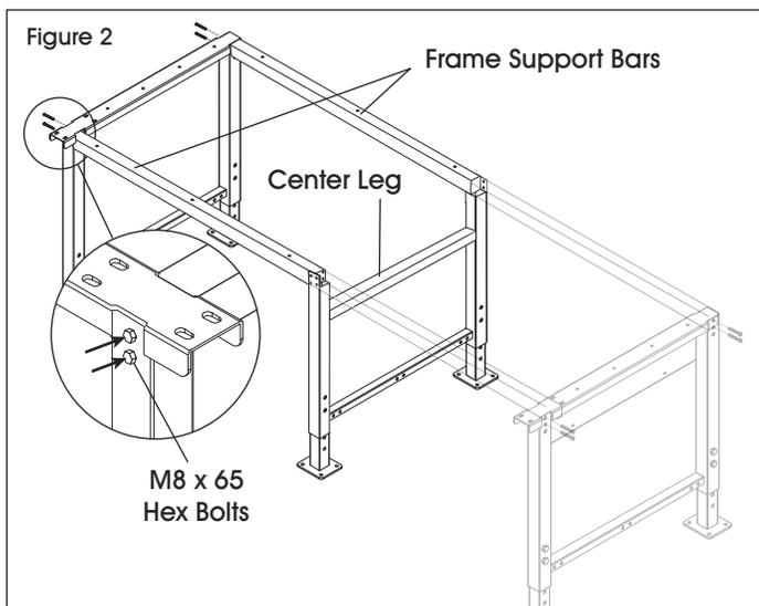
3. Place center leg support bar (6) between frame support bars (4) on top of the center leg. Fasten center leg support bar to frame support bars and center leg (1) with eight M8 x 65 hex bolts using a 13 mm wrench. (See Figure 3)
