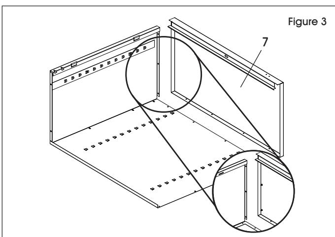
to the side panel on the unit. The threaded studs should go through the holes in the top flange of the side and fasten with three nuts. Attach the back to the top using four bolts and nuts. (See Figure 3)
