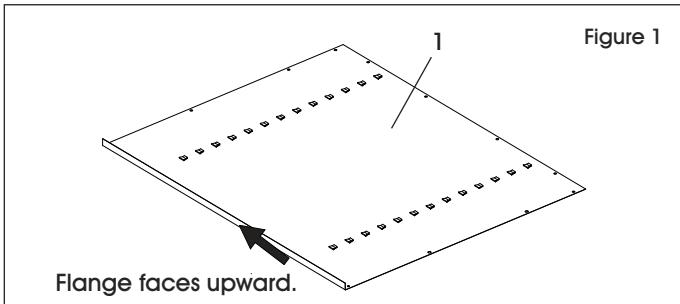
**NOTE:** When bolting the unit together, leave the bolts slightly loose until step 7, unless otherwise instructed.
