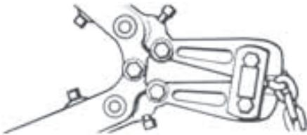
22B. Cutting Chain with a Bolt Cutter
