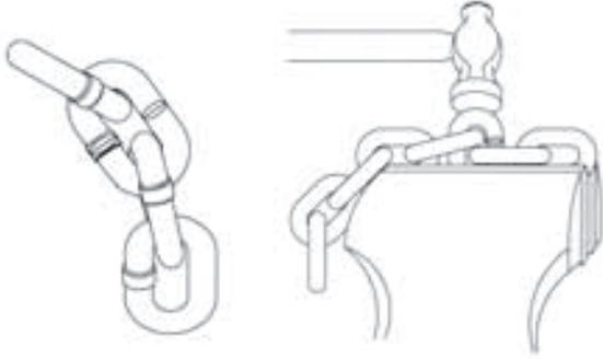
Figure 22A. Cutting Chain by Nicking Figure
