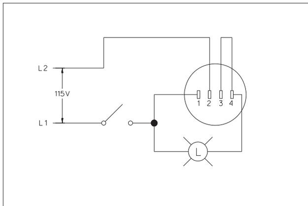
3. Close the switch to energize the 115-1-60/230-1-60 power supply. The light bulb will illuminate if the solid state reverse switch is not damaged. If the bulb fails to illuminate, the switch is damaged and must be replaced.
