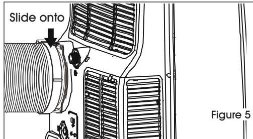
5. Affix adapter B into the window slider kit and seal. (See Figures 6 and 7)
