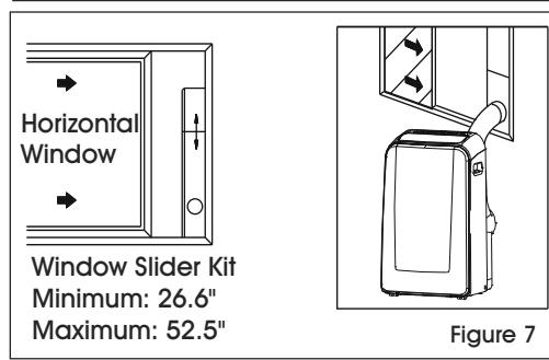
The hose can be extended from its original length of 15" up to 59", but it is the best to keep the length to the minimum required. Also, make sure that the hose does not have any sharp bends or sags. (See Figure 8)
