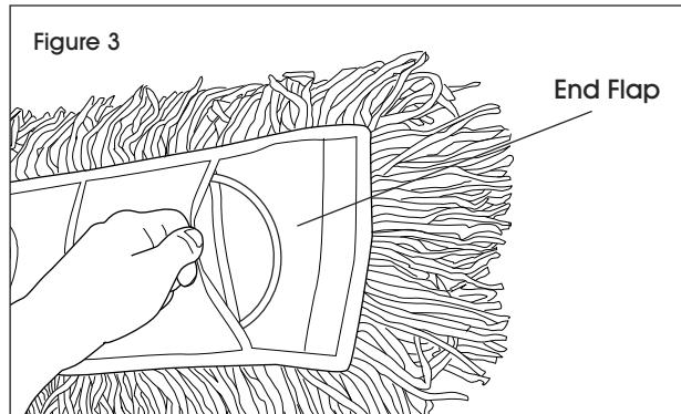
2. Slide the dust mop frame fully into the backing.
