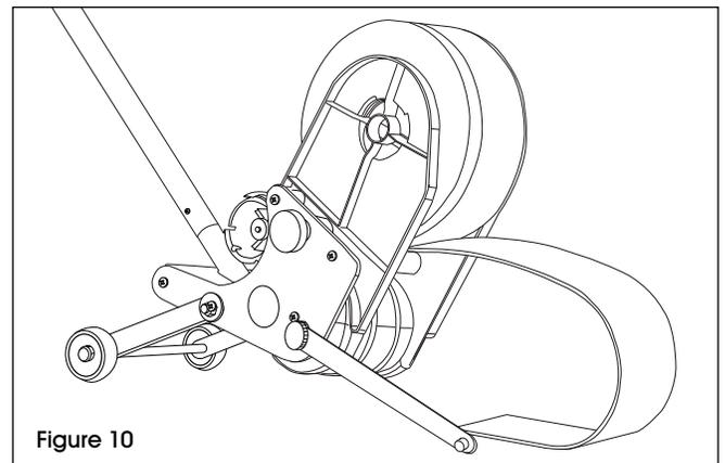
3. Pick up applicator and move it forward until tape is resting taut against roller wheel. (See Figure 11)
