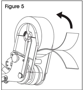
3. Before loading roll into applicator, ensure tape unrolls off bottom with adhesive side facing up, not over top of roll. (See Figure 3)
