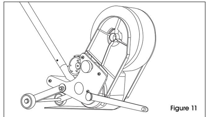
4. Press down on handle while pushing applicator forward to apply tape smoothly to floor.
