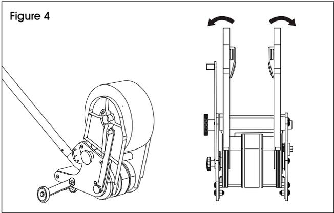
2. Turn large knob to adjust spacing between guide panels for either 2", 3" or 4" wide tape. (See Figure 2)
