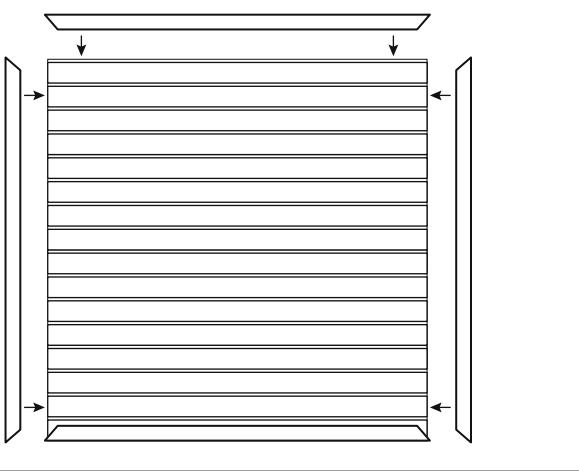
6. Slide three remaining miter cut J trim pieces into place. Adjust until corner pieces fit together. Tighten all screws to wall. (See Figure 6)
