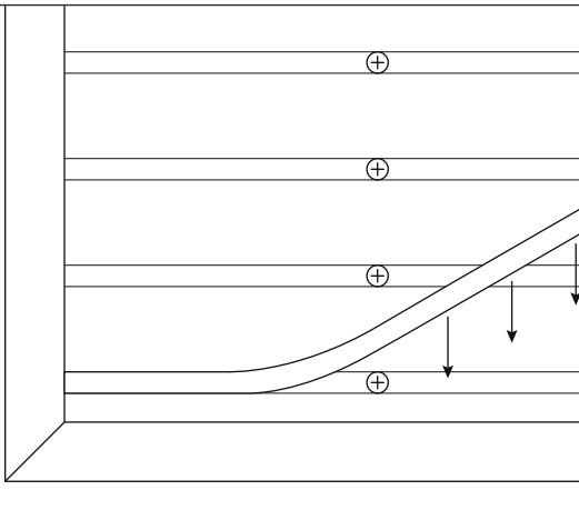
7. To completely hide screw heads, peel off backing of adhesive color strips and press into each slot of slatwall panels. (See Figure 7)
