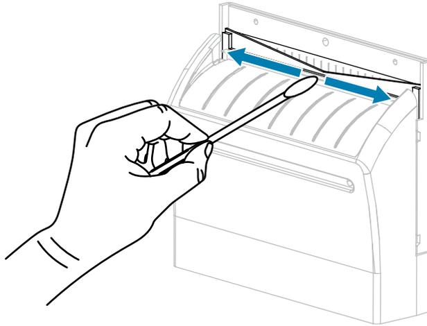
8. When the solvent has evaporated, soak a clean swab in a general-purpose, higher-viscosity silicone or PTFE oil lubricant.
