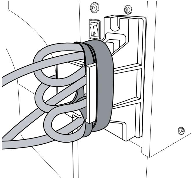
6. Plug the A/C power cord into an appropriate power outlet.
