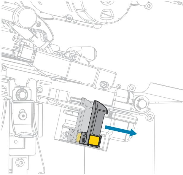
4. Push down the peel-off mechanism release lever to open the peel assembly.
