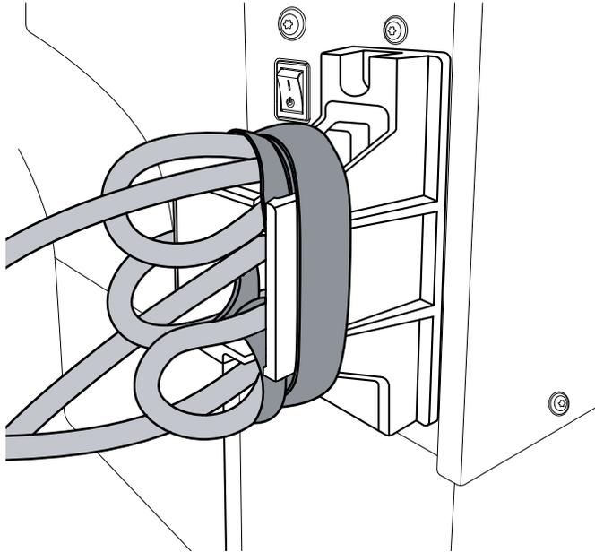
4. Plug the A/C power cord into an appropriate power outlet.
