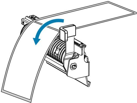
7. Thread the media into the slot below the peel assembly.
