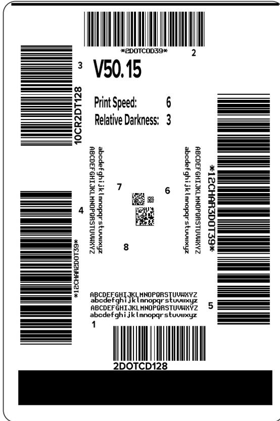
7. Examine the position of the label over the tear bar. If necessary, shift the position of the media over the tear-off bar after printing.
