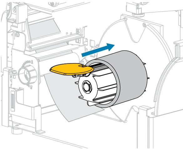
12. Wrap the media around the core as shown and turn the rewind spindle to tighten the media. Ensure that the edge of the media is flush against the backplate of the rewind spindle.
