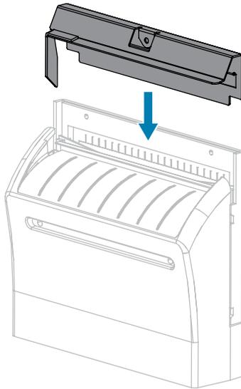
11. Secure it with the thumbscrew and lock washer that you removed earlier.
