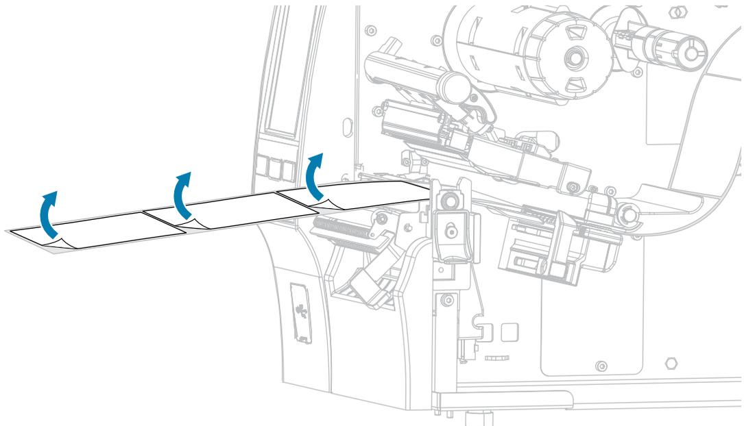
7. Feed the liner behind the peel assembly. Make sure that the end of the liner falls outside of the printer.
