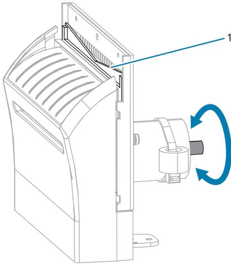
7. Using the swab from the Preventive Maintenance Kit (part number 47362), wipe along the upper cutting surface and the cutter blade. In place of the Preventive Maintenance Kit, you may use a clean swab dipped in 99.7% isopropyl alcohol. Allow the solvent to evaporate.
