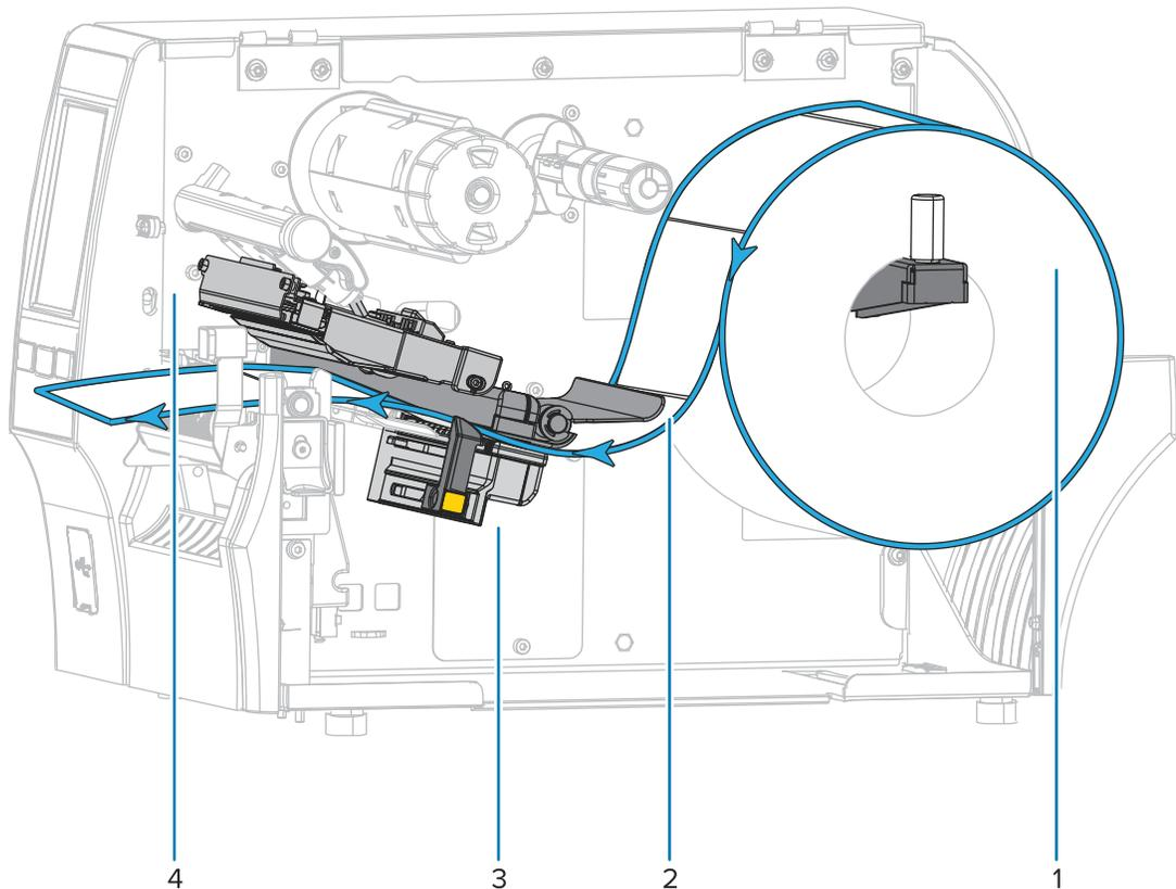
5. Extend approximately 18 in. (500 mm) of media out of the printer.
