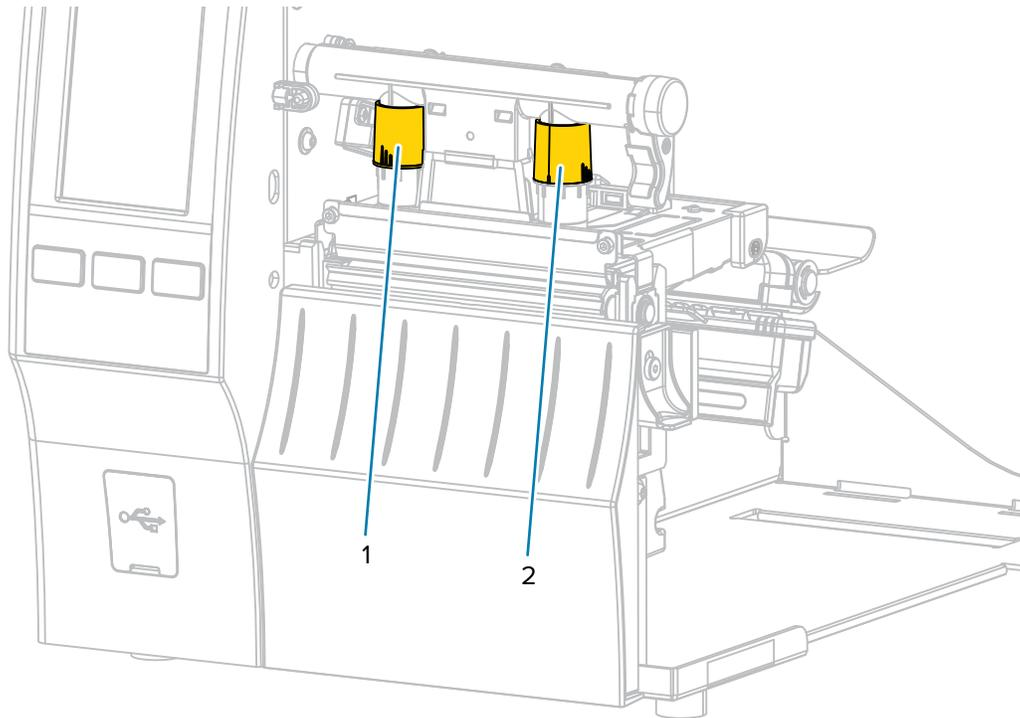
Begin with the pressure settings for your printer model and media width as specified in the following table, and make adjustments to the inside dial (1) and the outside dial (2) as necessary.
