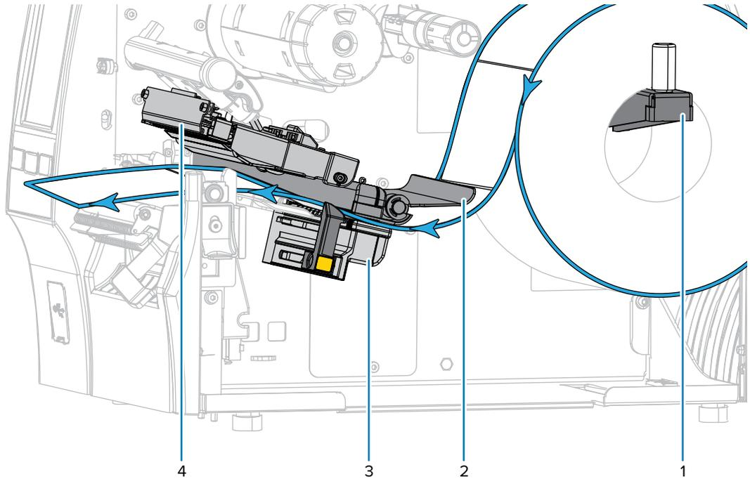
6. Extend approximately 18 in. (500 mm) of media out of the printer. Remove and discard the labels from this exposed media, leaving just the liner.
