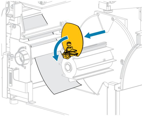
11. Slide an empty core onto the rewind spindle.
