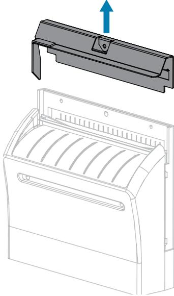
6. If necessary, rotate the cutter motor thumbscrew to fully expose the V-shaped cutter blade (1).
