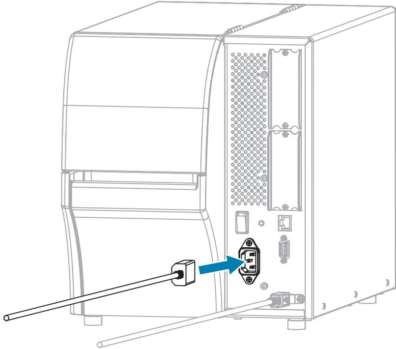
3. Plug the A/C power cord into an appropriate power outlet.
