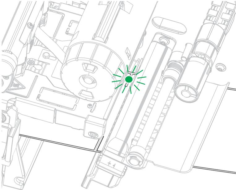
3. If necessary, slide the media sensor horizontally using the media sensor adjustment.
