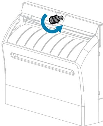
5. Remove the cutter shield.
