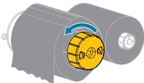
The ribbon release bars pivot down, easing the spindle's grip on the used ribbon.
