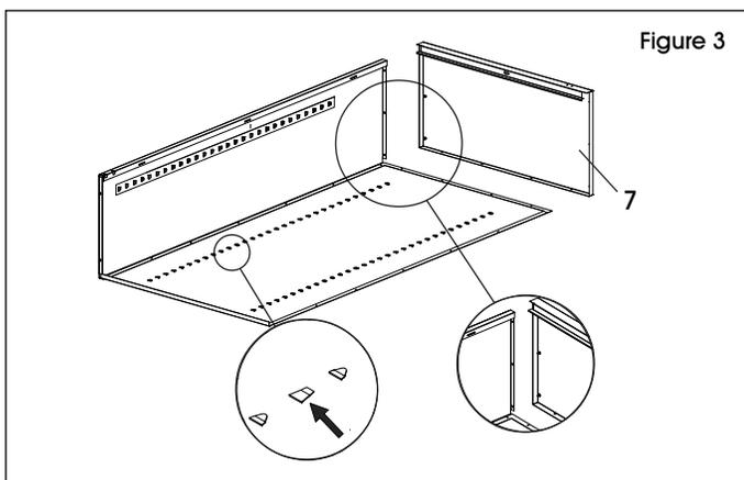
4. Attach the right side (3) to the back as done in step 2. Ensure the flange is around the back and that the lances on the shelf adjustment strips are pointed in the same direction as those on the back and left side. Push the side panel up so the studs in the top go through the holes in the top flange of side and fasten with three nuts. (See Figure 4)
