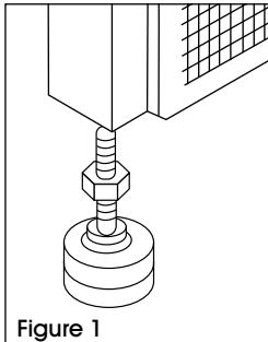
3. Tighten leveling glide and nut using wrench.
