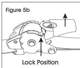
**NOTE:** Handle must be in line with direction of pull to achieve working load limit. (See Figure 3)
