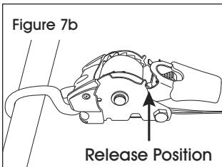
7. When in release position, unhook the tie-down from anchor points and press red button to retract. (See Figure 8)
