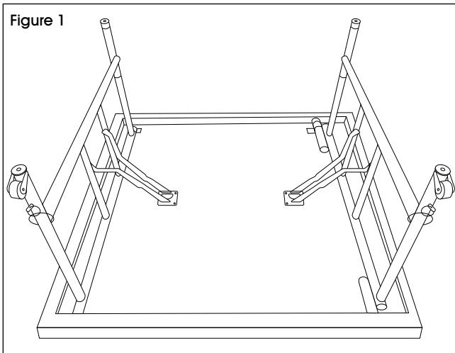
2. To adjust platform height, pull out steel pin completely from leg and loosen black knob clockwise one turn. (See Figure 2)
