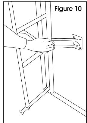
2. Fold leg assembly against the underside of stage platform. (See Figures 11-12)
