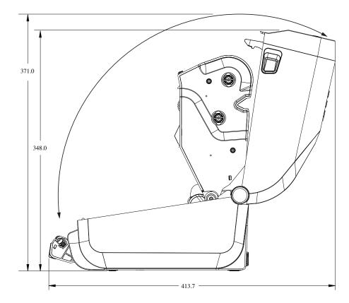
Figure 23 ZD421 / ZD621 Thermal Transfer Models – Dimensions for Printer with Cutter Option Installed
