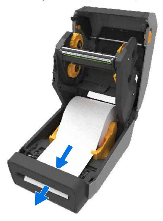
2. Close the printer. Press down until the cover snaps closed.
