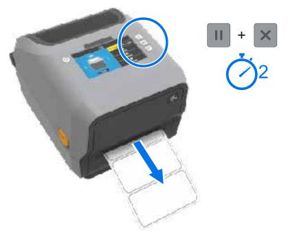
The printer feeds and measures a few labels and adjusts media sensing levels. When it completes measuring, the STATUS indicator lights solid green.
