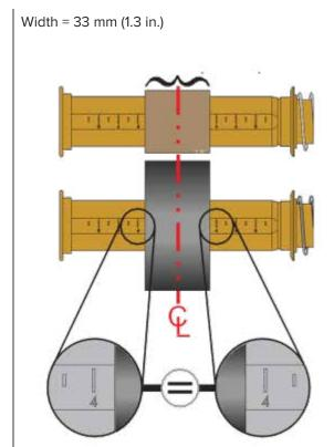
3. Place the adapter with an empty core on the take-up spindles and the adapter with the ribbon roll on the lower supply spindles. The right side of the core adapter fits on the cone-tip on each of the spring-loaded right-side spindles. Continue pushing the adapter onto right-side spindle and swing
