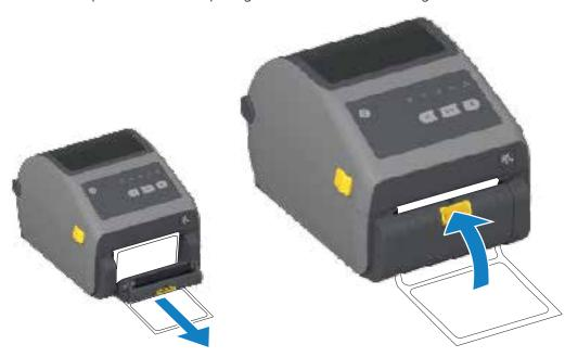
5. Press and release FEED (Advance) one or more times until a label is presented for removal.
