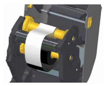
**6.** Turn the ribbon take-up hub with the top moving towards the rear to remove slack from the ribbon. Rotate the hub to finish aligning the take-up ribbon position with the supply-ribbon roll. The ribbon should be wound, at a minimum, one-and-a-half times around the take-up ribbon core.
