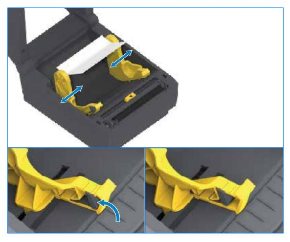
**6.** Insert the media through the slot at the rear of the printer, and place the media between the media guide and roll holders.
