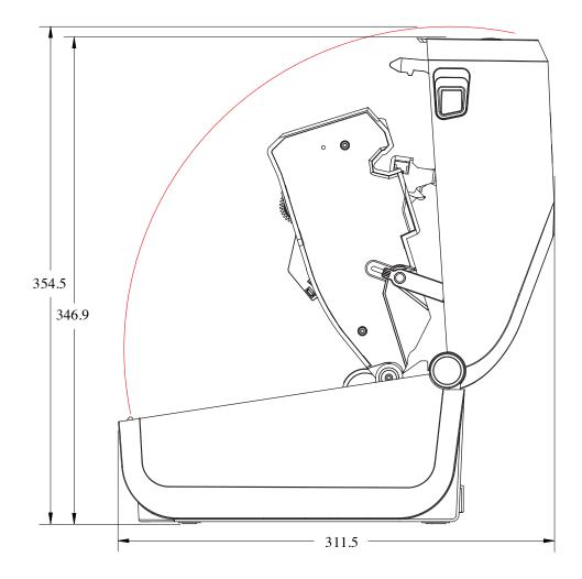
**Figure 31** ZD421C (Ribbon Cartridge Thermal Transfer) Printer Models – Dimensions of the Printer with the Label Dispenser Option Installed
