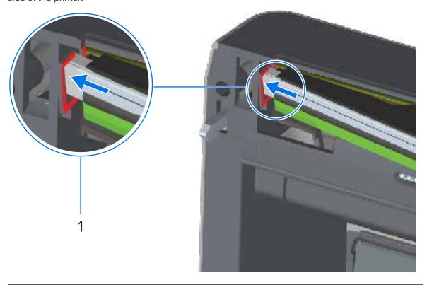
e) Align the spring wire notch on the backside of the printhead to the spring wire. Push the right side of the printhead into the printer until the latch locks the right side of the printhead into the printer.
