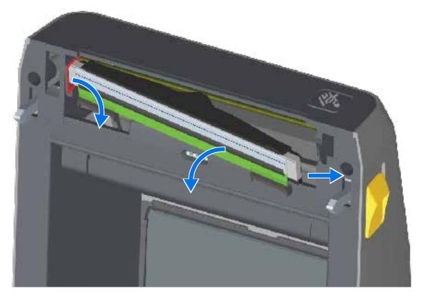
**f)** Gently but firmly pull the two printhead cable bundle connectors off the printhead. Then pull the ground wire off the printhead.
