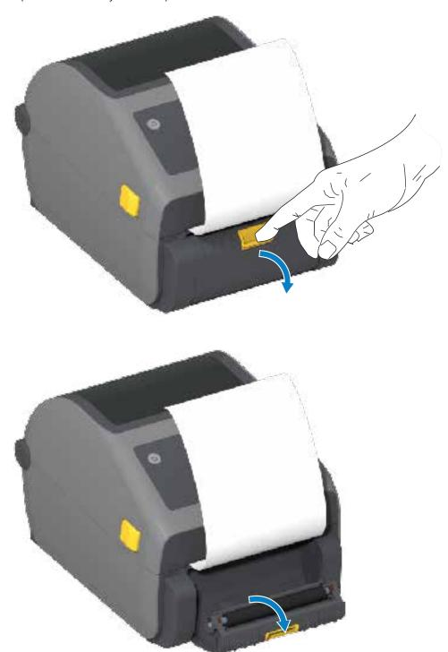
**3.** Insert the label liner between the dispenser door and the printer body.
