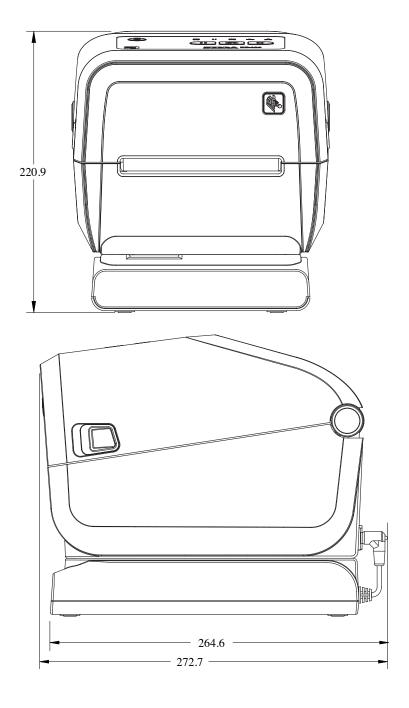
**Figure 35** ZD421C (Ribbon Cartridge Thermal Transfer) Printer Models – Dimensions of the Printer with Attached Power Supply Base and Battery
