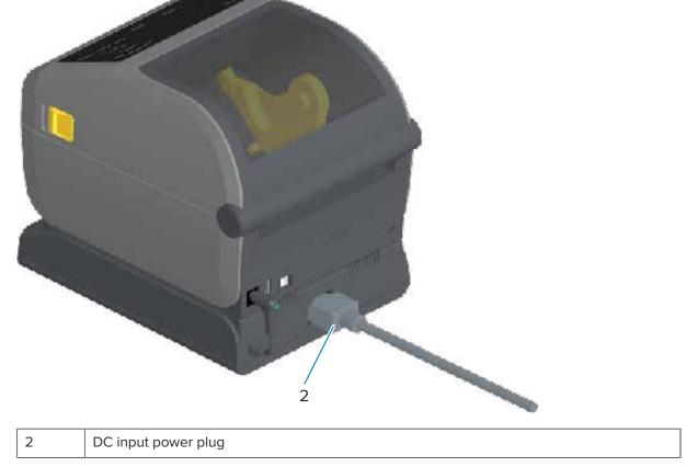
**6.** Re-connect the AC power cord to the printer power base.
