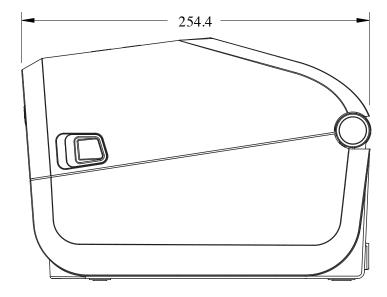
**Figure 30** ZD421C (Ribbon Cartridge Thermal Transfer) Printer Models – Dimensions of the Standard Printer with Cover Open
