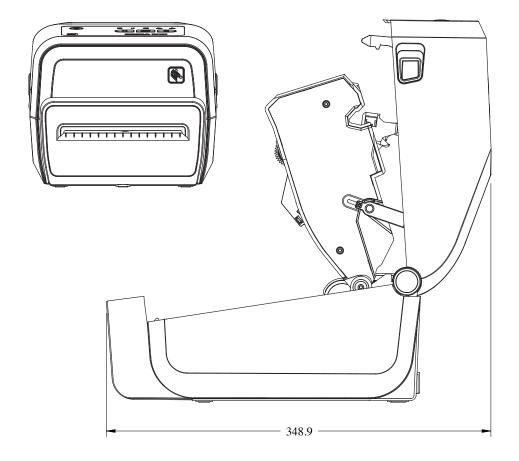
**Figure 34** ZD421C (Ribbon Cartridge Thermal Transfer) Printer Models – Dimensions of the Printer with Attached Power Supply Base
