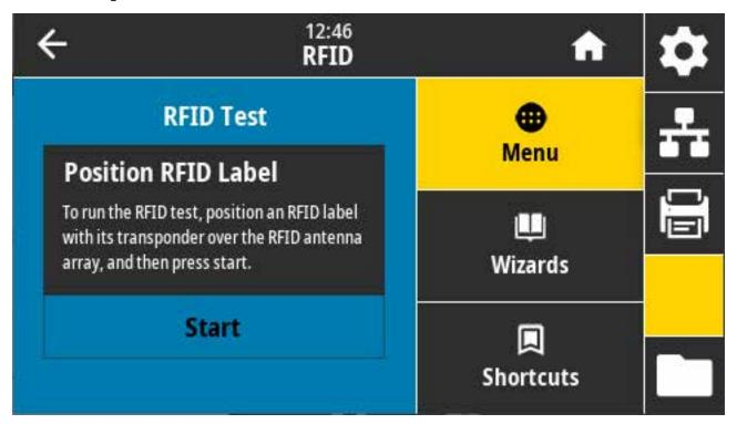
To test an RFID label, position an RFID label with its transponder above the RFID antenna array. Then touch **Start**.
