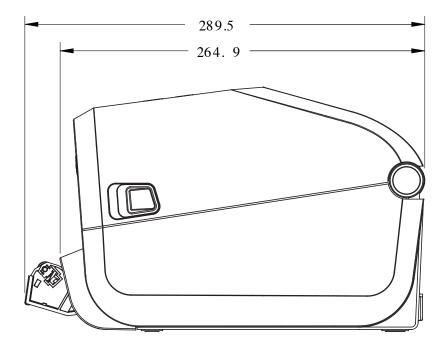
**Figure 32** ZD421C (Ribbon Cartridge Thermal Transfer) Printer Models – Dimensions of the Printer with the Label Dispenser Option Installed and Cover Open
