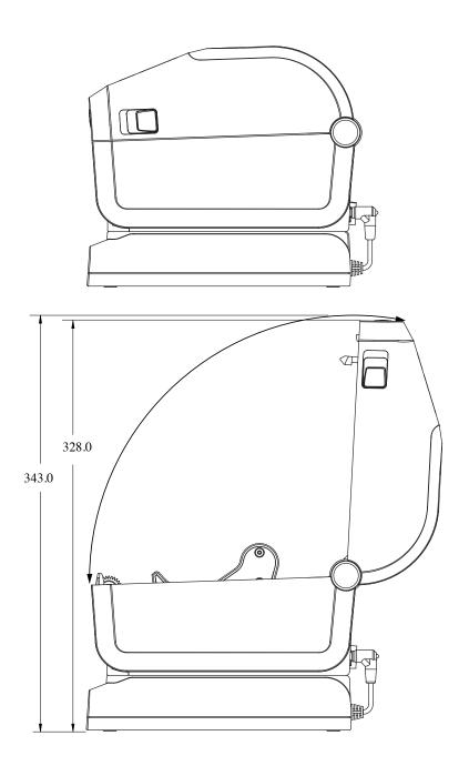
**Figure 18** ZD421/ZD621 Direct Thermal Printer Models – Dimensions of the Printer with the Attached Battery Base and Battery
