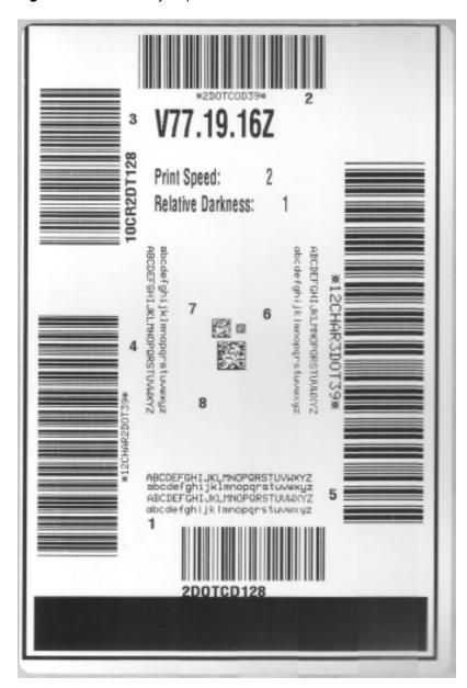
The speed at which labels are printed during this print quality test depends on the dot density of the printhead.
