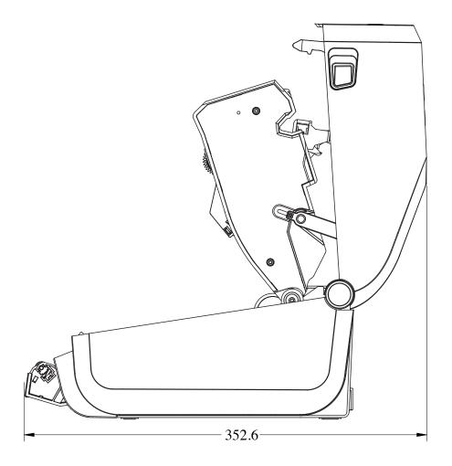
**Figure 33** ZD421C (Ribbon Cartridge Thermal Transfer) Printer Models – Dimensions of the Printer with the Cutter Option Installed
