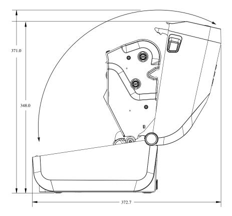
**Figure 22** ZD621 / ZD421 Thermal Transfer Models – Dimensions for Printer with the Label Dispenser Option Installed
