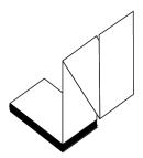
Non-continuous media that comes folded in a rectangular stack and folded in a zigzag pattern. Fanfold media is either gap-notch media or black mark media, meaning it uses black marks or notches to track media format positioning.
