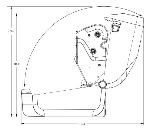
**Figure 24** ZD421 / ZD621 Thermal Transfer Models – Dimensions for Printer with the External Battery Plugged In
