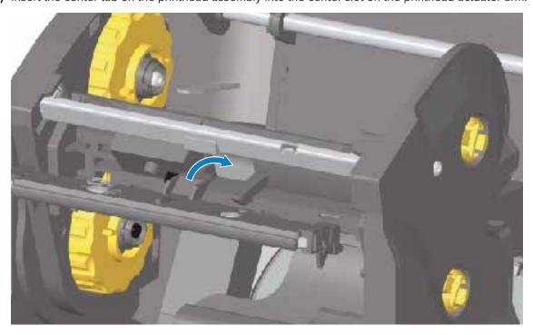
**d)** Insert the left side tab of the printhead assembly into the recessed slot on the left side of the printhead actuator arm.
