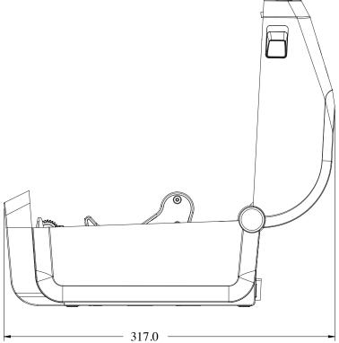
**Figure 17** ZD421/ZD621 Direct Thermal Printer Models – Dimensions of the Printer with the Power Supply Base Plugged in
