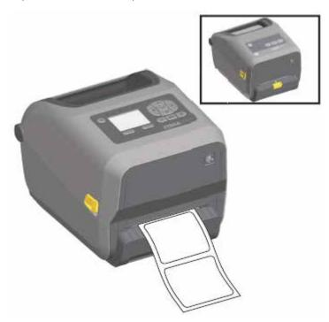
**2.** Lift the liner over the top of the printer, then open the door by pulling the gold latch in the center of dispenser door away from the printer.
