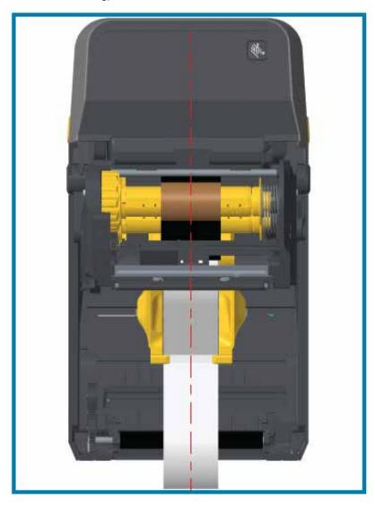
**5.** Attach the ribbon to the take up core. If your media does NOT have an adhesive strip on the ribbon leader as Zebra-manufactured ribbon does, use a thin strip of tape to secure the ribbon to the take-up core. Align the ribbon so that it will be taken straight onto the core.
