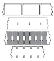
• Black mark media uses pre-printed black marks on the back side of the media to indicate label separations.
