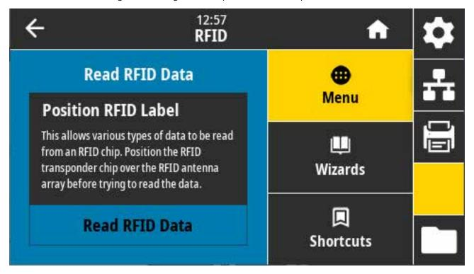
To read and display the information stored on an RFID tag, position the RFID label with its transponder over the RFID antenna, then touch **Read RFID Data**.
