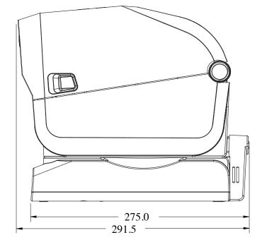
**Figure 27** ZD421 / ZD621 Thermal Transfer Models – Dimensions for Printer with Power Supply Base Attached and Printer Open
