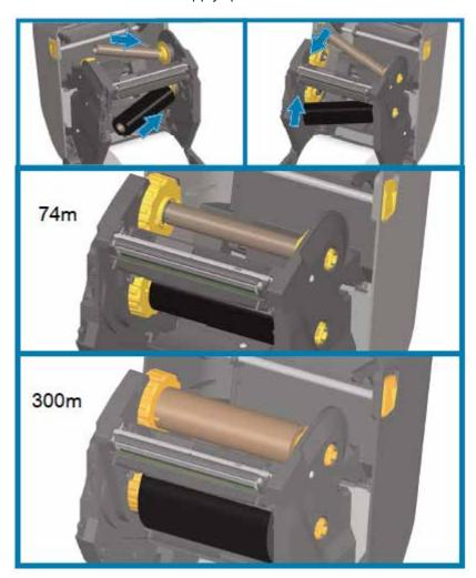
**4.** Attach the ribbon to the take-up core. Use the adhesive strip on new rolls; otherwise, use a thin strip of tape. Align the ribbon so that it will be taken straight onto the core.
