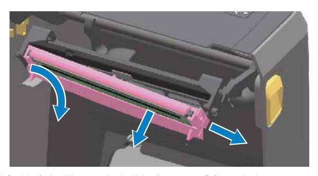
e) Gently but firmly pull the two printhead cable bundle connectors off of the printhead.
