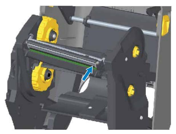
**f)** Verify that the printhead moves up and down freely when pressure is applied and remains locked when released.
