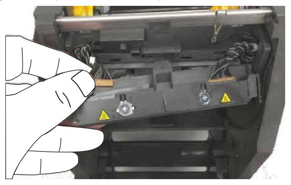
c) Insert the center tab on the printhead assembly into the center slot on the printhead actuator arm.
