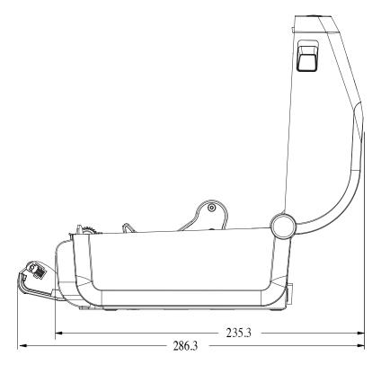
**Figure 16** ZD421/ZD621 Direct Thermal Printer Models – Dimensions of the Printer with the Cutter Option Installed
