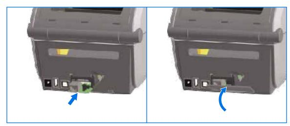
**2.** Align the bottom of the Ethernet port's door cover to the bottom lip of the module access opening, then swing the door up and snap the cover closed.
