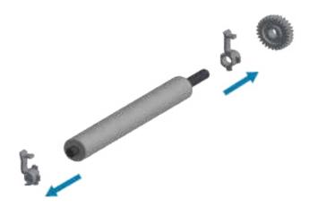
**6.** To clean a regular platen, use alcohol moistened swab or lint-free cloth very lightly moistened with 99.7% pure, medical-grade isopropyl alcohol using the steps below.
