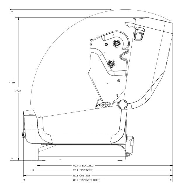
**Figure 26** ZD421 / ZD621 Thermal Transfer Models – Dimensions for Printer with Power Supply Base Attached
