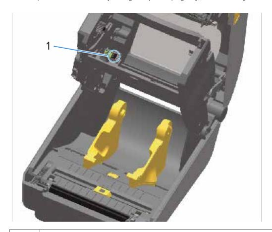
1 Ribbon cartridge sensor contact pins
