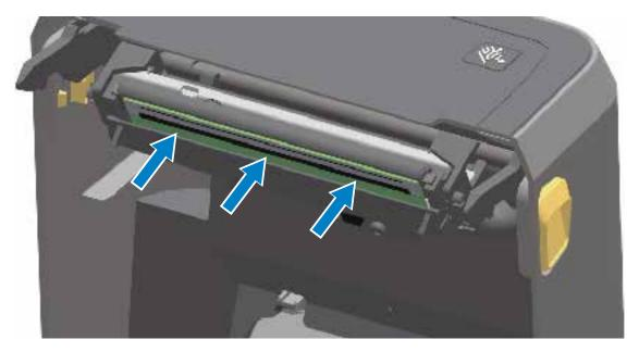
**g)** Clean the printhead by using a new cleaning pen to wipe body oils (finger prints) and debris off the printhead. See Cleaning the Printhead on page 272.
