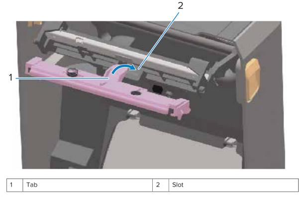
**d)** Insert the left side tab of the printhead assembly into the recessed slot on the left side of the printhead actuator arm.
