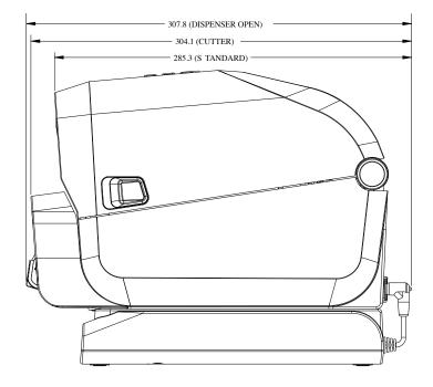
**Figure 25** ZD421 / ZD621 Thermal Transfer Models – Dimensions for Printer with External Battery Plugged In and with Printer Open
