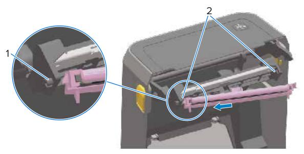
**e)** Push the right side of the printhead into the printer until the latch locks the right side of the printhead into the printer.
