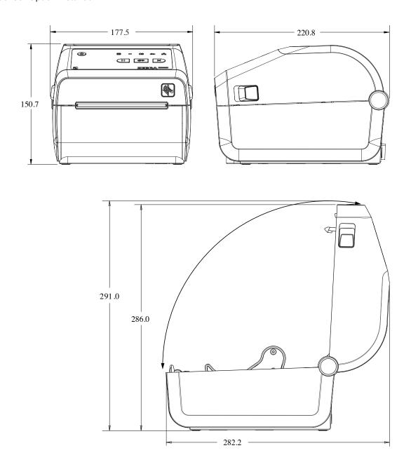
**Figure 15** ZD421/ZD621 Direct Thermal Printer Models – Dimensions of the Printer with the Label Dispenser Option Installed
