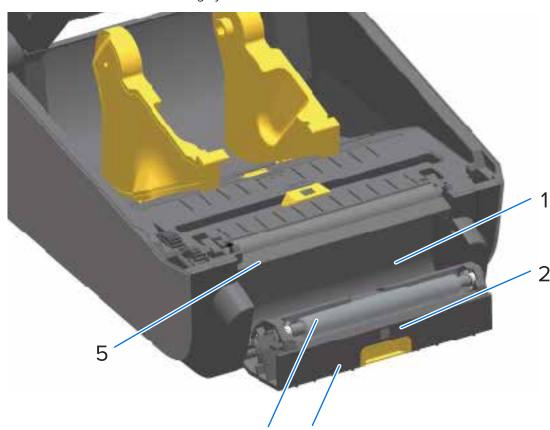
**5.** Clean the sensor window thoroughly until it is clear of streaks and residue.
