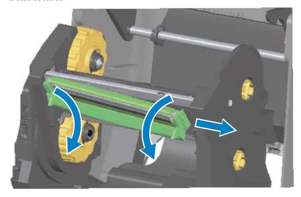
d) Gently but firmly pull the two printhead cable bundle connectors off of the printhead.
