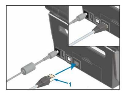
1 Ethernet cable (RJ-45 connector)
