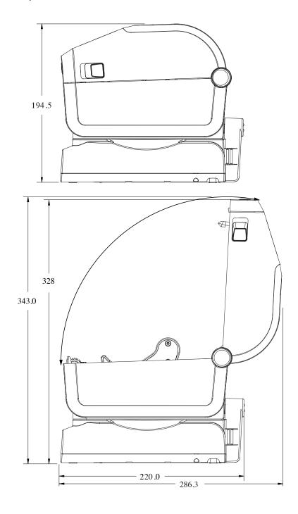
**Figure 19** ZD621 Direct Thermal Printer (Healthcare Models Only) with Locking Media Cabinet – Dimensions
