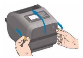
**2.** Open the media roll holders. Orient the media roll so that its printing surface will face up as it passes over the platen (drive) roller. Pull the media guides open with your free hand and place the media roll on
