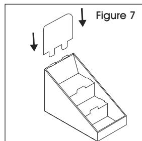
4. Place insert in display. The tabs on the side of the insert should align with and snap into the slots on the side panels of the display. (See Figure 4)
