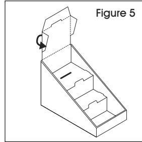
2. Fold over side flaps and front lip. Lock them into the slots at the display bottom. (See Figure 2)
