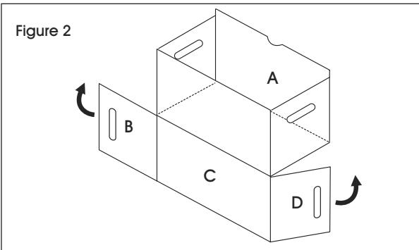
3. Fold sides B, C and D up to form bottom of carton. (See Figure 3)
