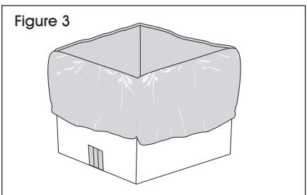
5. Pour a minimum 1.66" even layer of Grade 4 vermiculite into the bottom of the poly bag.
