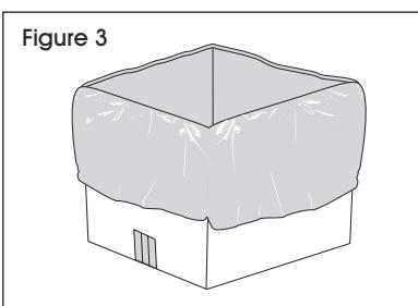
5. Pour a minimum 2.89" even layer of Grade 4 vermiculite into the bottom of the poly bag.
