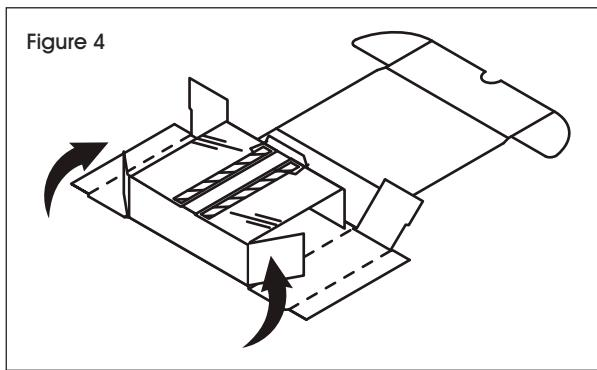
2. Fold both tension flaps (A) with equal force down and under panel (C). (See Figure 2)
