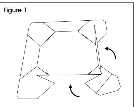
2. Fold end tabs on each long panel inward so the two tabs meet in the middle. (See Figure 2)
