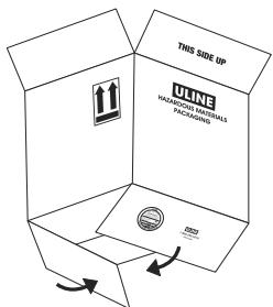
3. Seal bottom of carton with three parallel strips of 2" wide (2.6 mil) polypropylene tape (Uline Model # S-14564). The tape must overlap 0.5" side to side and extend 3" over each end of the carton. (See Figure 2)
