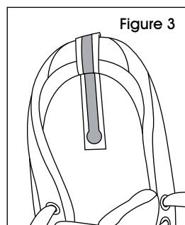
4. Ensure the grounder stays under the foot when the shoe is on. (See Figure 4)
