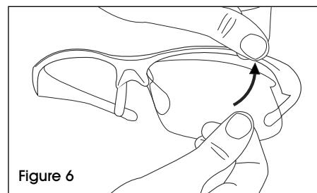
2. Push the left lens upward into the frame at the nasal area first, then snap the lens in at the temple. (See Figures 7-8)
