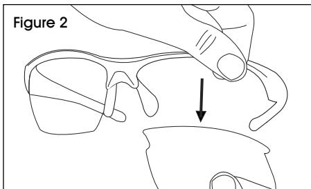
2. Unhook the left lens at the temple first by pulling the frame and lens away from each other simultaneously. (See Figures 3-4)
