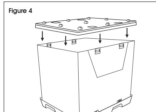
5. To secure, slide all four clips on lid into locked position. (See Figure 5)
