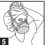
1. Without touching the respirator, slowly lift the bottom strap from around your neck up and over your head. Then lift off the top strap. Store or discard according to your facility's infection control policy. Dispose of used product in accordance with applicable regulations.
