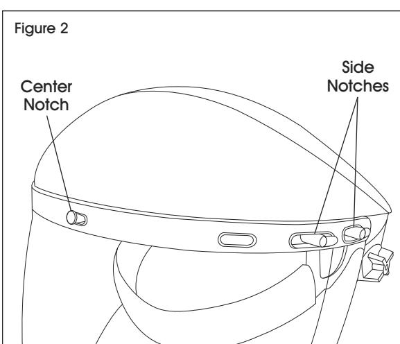
4. Turn side notches up or down to secure face shield. (See Figure 4)
