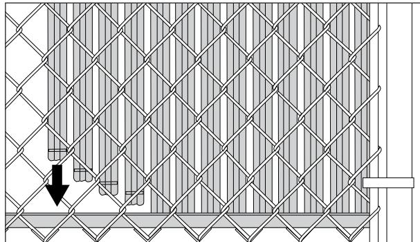
3. Push vertical slat into bottom channel to lock in place. (See Figure 3)
