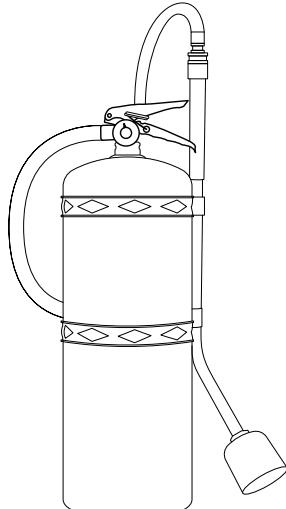
2. Attach handle to opposite end of hose with built-in quick-connect coupler. (See Figure 2)
