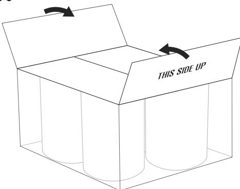
8. Seal top of carton down the center seam with one strip of 2" wide (2 mil) polypropylene tape (Uline model # S-423). Tape must extend 3" over each end of the carton. (See Figure 6)
