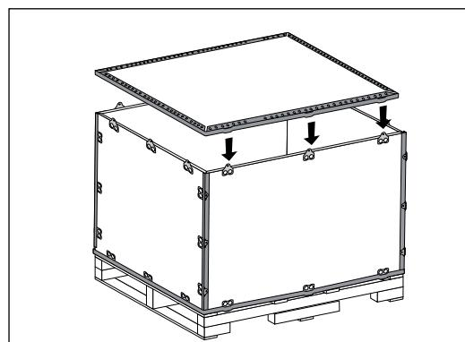
2. Secure short panels to base and sides of long panel.
