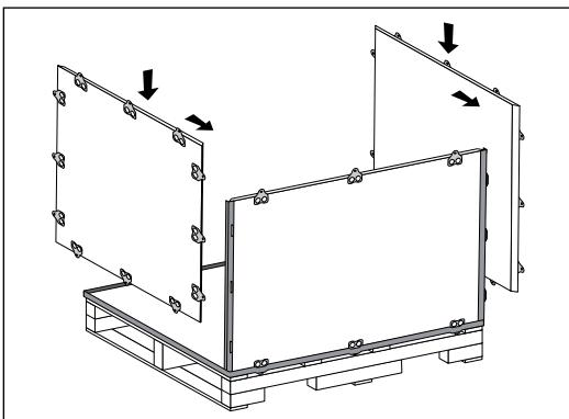
5. Bend back all tabs using a screwdriver or a hammer.
