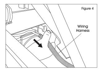
Remove the wiring harness from the batteries starting with the outermost cables that come from the table. (See Figure 5)
