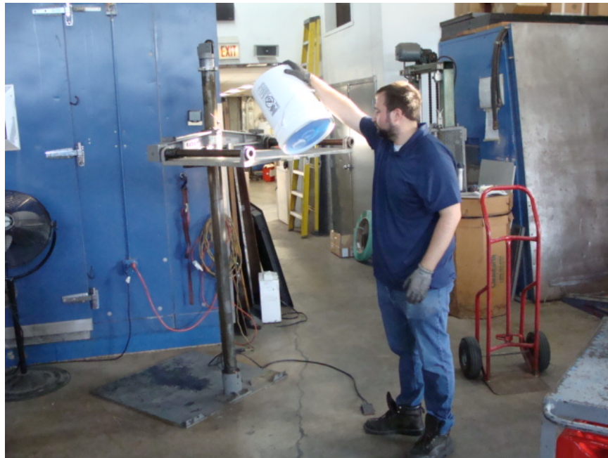
Photo No. 1 - Top Diagonal Drop Setup
