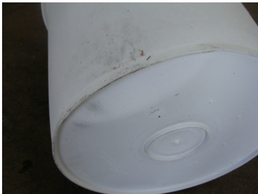
Photo No. 6 – Slight Distortion on the Drum After the Flat Side Drop
