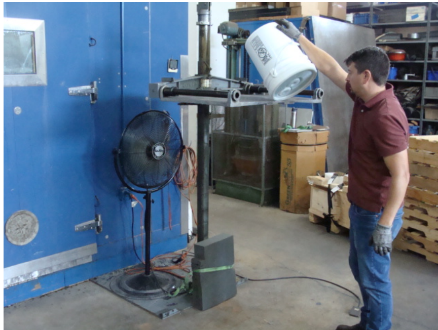
Photo No. 1 - Top Diagonal Drop Setup
