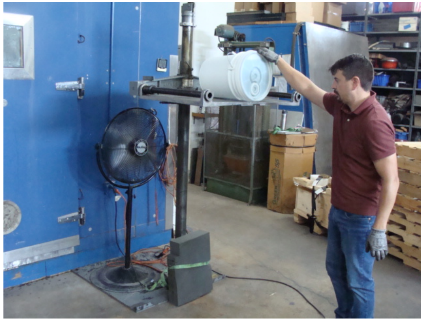
Photo No. 3 - Flat Side Drop Setup
