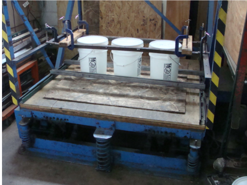
Photo No. 9 –Vibration Test Setup
