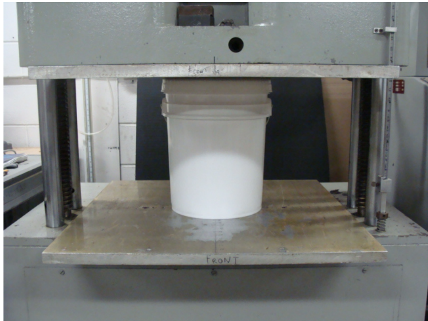
Photo No. 10 –Stacking Test Setup
