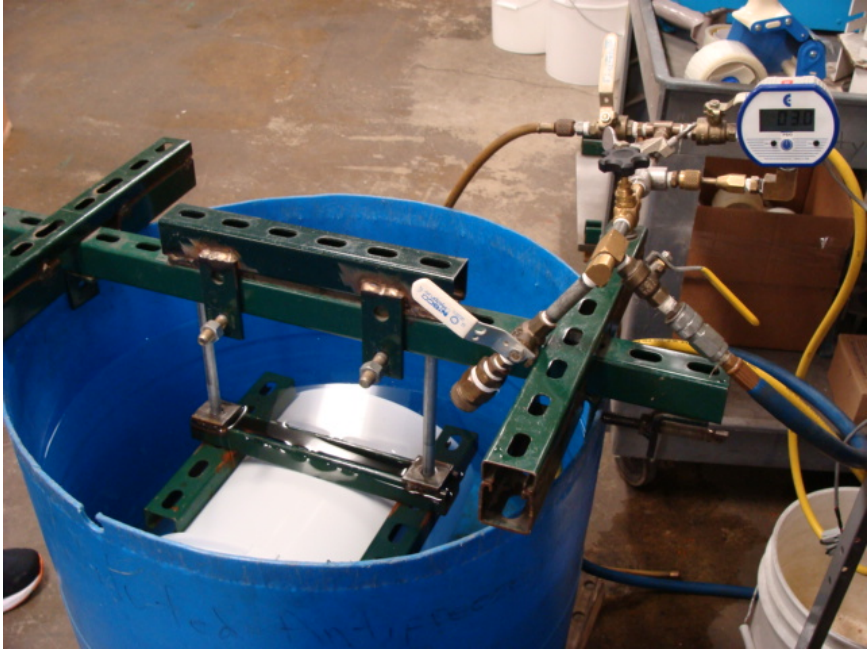
Photo No. 7 - Leakproofness Test Setup
